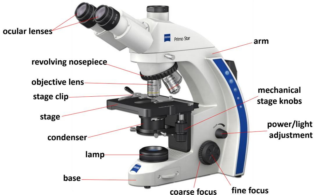
**OCULAR LENS (eyepiece)** – Your microscope will have either one (monocular) or two (binocular) **ocular lenses**. These are the lenses you will look through when examining a specimen with the microscope. Take a look at the side of your ocular lens and you will notice a label of “10X”. This indicates that each ocular lens magnifies the image by a factor of 10 or 10X.
